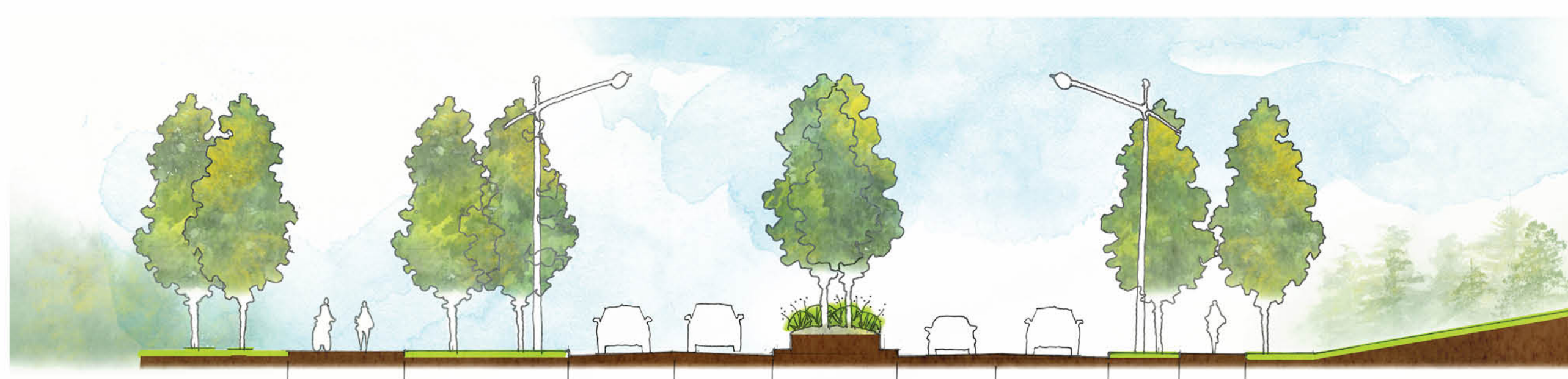
The reconstructed Almond Street would typically include two lanes, as well as turn bays when needed, in each direction.
