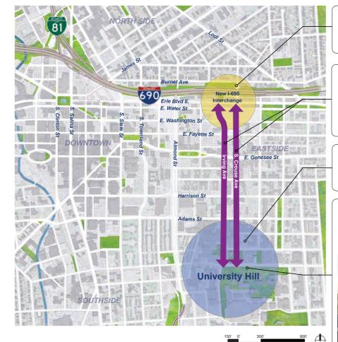
The new interchange would provide an access point to I-690 and to BL 81 (via I-690) to and from the north, east, and west; would reduce reliance on Almond Street; and would restore the missing street grid on Irving Avenue.
